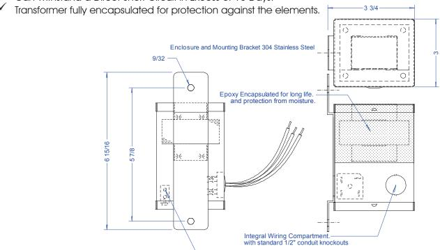
Power supply is designed to be used in conjunction with a dimmer. If a dimmer is not utilized, check output voltages at connection to LED fixture to insure DC voltage does not exceed rating of fixture.
